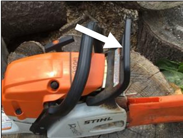
Figure 4. A chain brake/kickback protection device.
