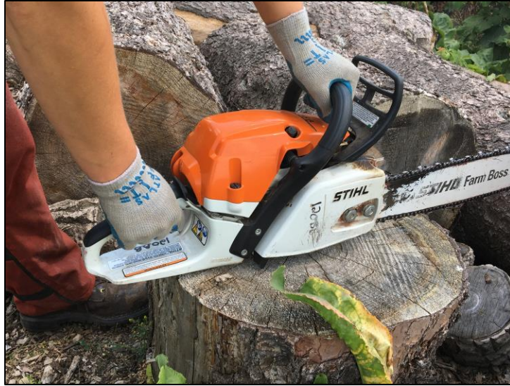
Figure 7. Proper hand grip for top-handled chain saw.
