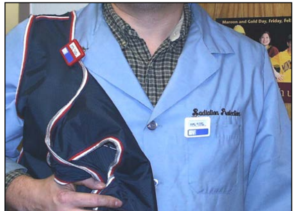
Dual dosimeters (body & collar for X-ray fluoroscopy). Wear the body dosimeter at belt or chest level under the lead apron, and wear the collar dosimeter at the collar on the outside of the lead apron.
