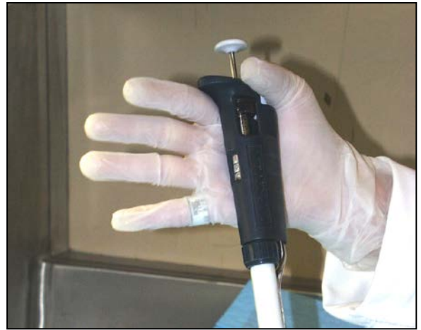
Ring dosimeter. Wear on finger closest to the radiation source with name label rotated toward the source.
