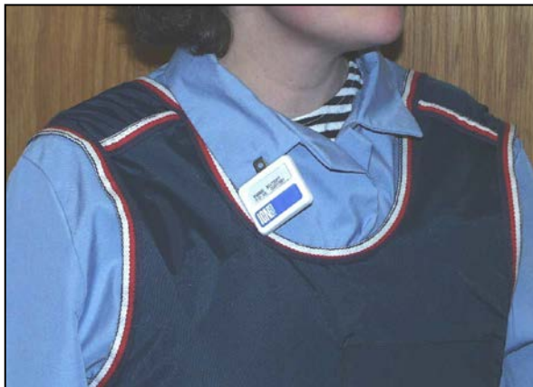
Body dosimeter with lead apron. Wear the body dosimeter at the collar outside of the lead apron.
