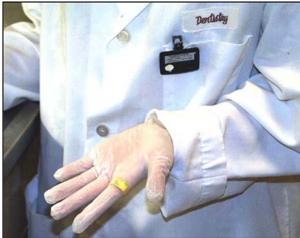
Body dosimeter. Wear on trunk of body at chest level with name plate facing outward.
