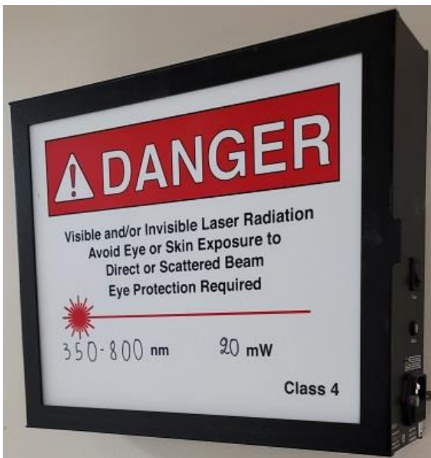
Fig 5. Example of a lighted sign operated either manually or automatically when a laser system is activated.
