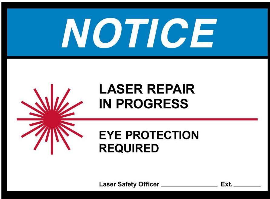
Fig. 4. Signage used when a laser or laser system is undergoing maintenance. Often displayed when a normally enclosed laser system is undergoing repair or maintenance and safety interlocks, protective panels, etc. are removed allowing for the possibility of laser radiation exposure.
