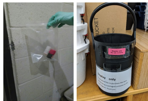
Figure 1: Secondary containers for small quantities (left) or low hazard (right)
