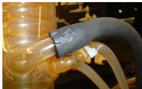
Figure 5: Cracking Rotovap condenser hose that has no securing tie
