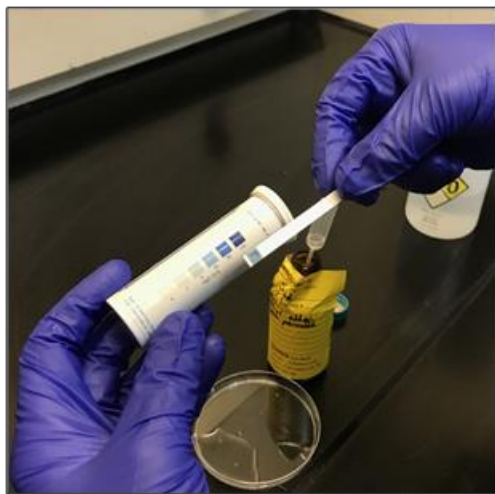
Figure 6: Testing for Peroxides
