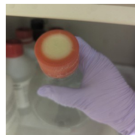
Fig. 3. A nitric acid bottle with it's orange cap discolored by a pale yellow circle in the middle, indicating corrosion of the cap.
